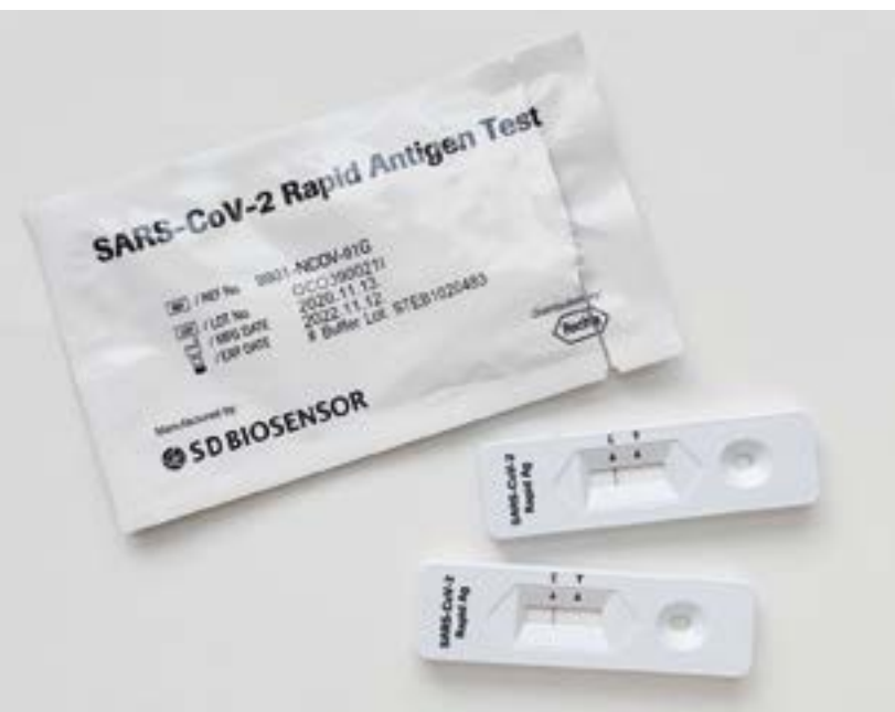
Figure 2. One of the most popular and well-known optical biosensors is the lateral-flow assay (LFA) test. These devices have been broadly used by the society for decades, for example for pregnancy detection and, more recently, for self-diagnosis of COVID-19.
