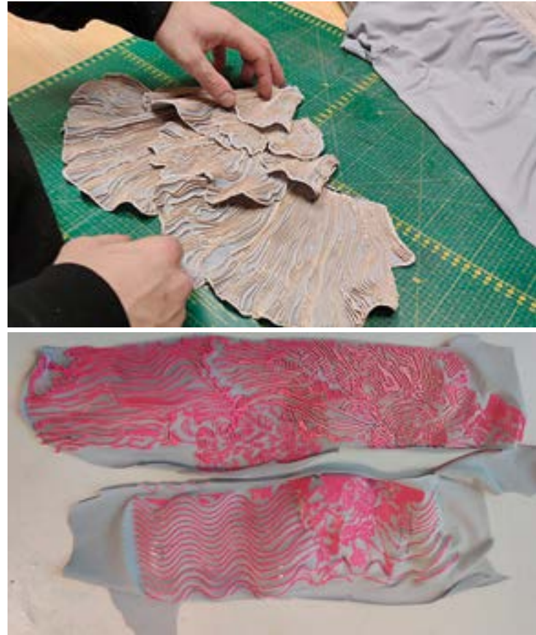
Figure 7. MonkeyFab's 3D printed textiles, from Patryk Wojciechowski's original design.
